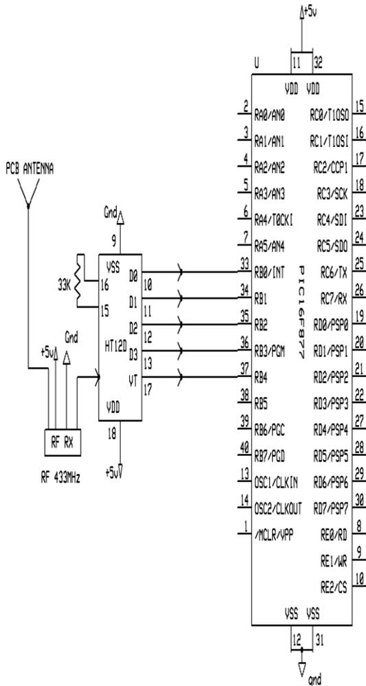
**RF MODULE INTERFACING WITH MICRO CONTROLLER**
