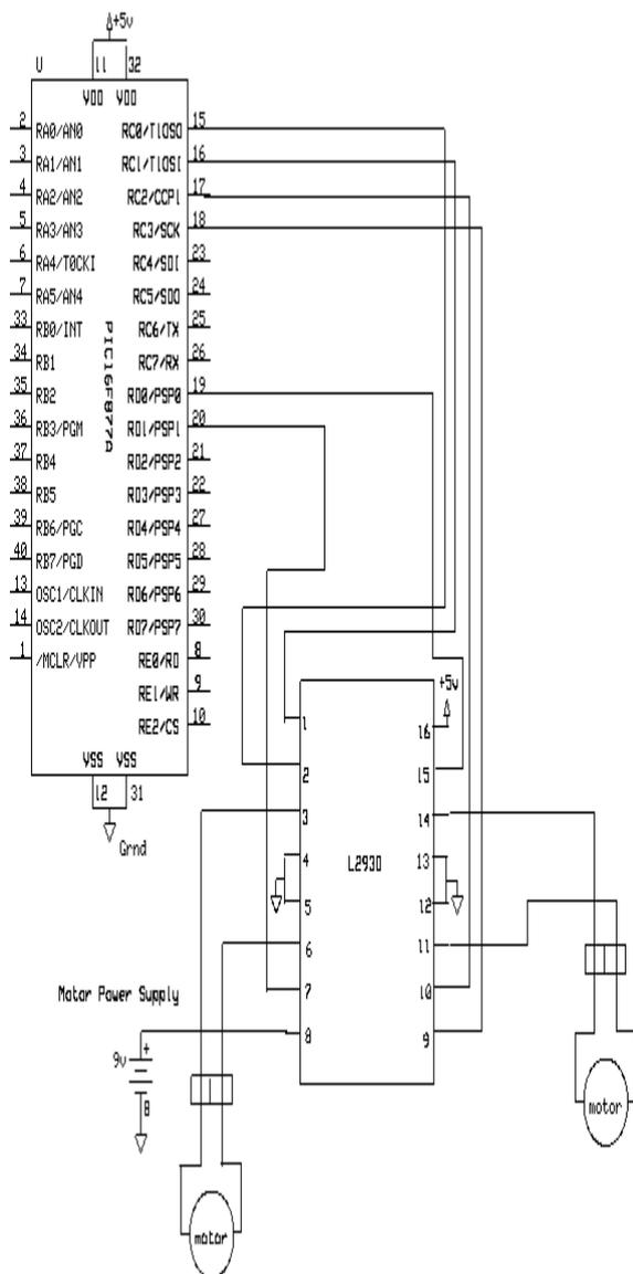
**MOTOR DRIVER INTERFACING WITH MICRO CONTROLLER**
