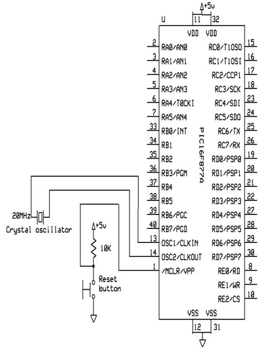
**CRYSTAL OSCILLATOR INTERFACING WITH MICRO CONTROLLER**
